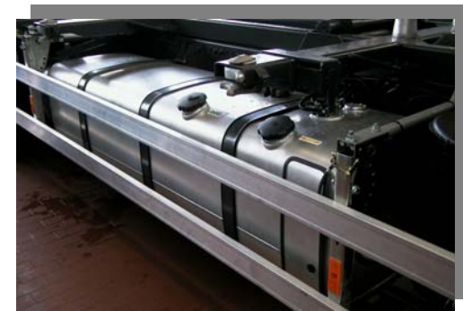
Urea dosing Unit and Integrated Urea/Diesel Tank
